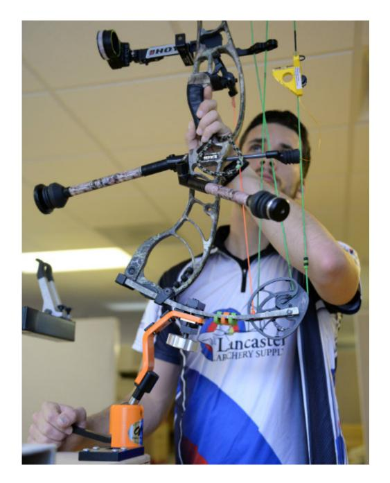
Next place a level on top of your scope housing, so it's parallel to the sight bar. If it's possible for you to do so, spin your scope until the bubble is centered. Now you've set the first axis. (Many sights won't have an adjustment for this axis, and will already be leveled by the manufacturer.)
