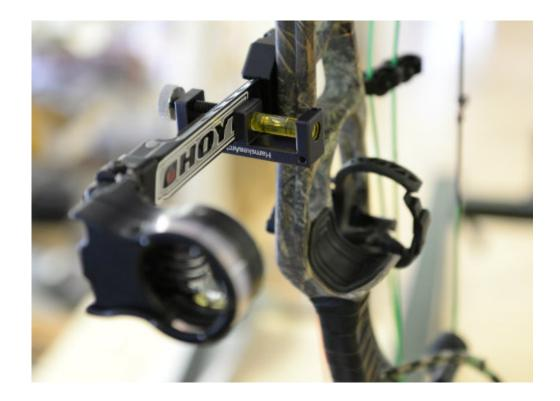
And so look at the level that's in the scope housing, and which is also perpendicular to the sight bar. Assuming your sight has the capability, adjust the scope using the second-axis adjustment screws until that bubble hits the center, too. When it does, you've leveled the second axis.
