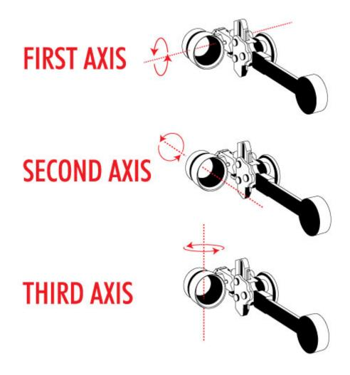
The first axis runs from left to right in front of you, parallel to the ground. If you have a scope around your sight, then this axis would allow it to spin bottom over top.
